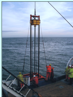
Vibro core sediment samples collected from the IMAGIN study Areas 1-4 (in total 36 cores = 128m of sediment recovered).
